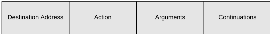
Figure 2: Structure of a HPX Parcel. A parcel has four components: the destination address; the action, which is the method/function to execute at the destination; the arguments for the function; and optional continuations.
